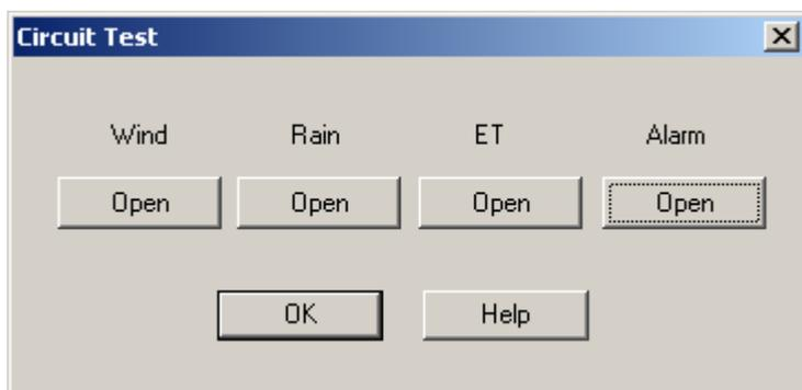
Pressing the Circuit Test button puts the Irrigation data logger into Circuit Test mode. In this mode, all other functions of the data logger cease. Do not press this button unless you wish to perform a test because it may disrupt the behavior of your Irrigation system.
