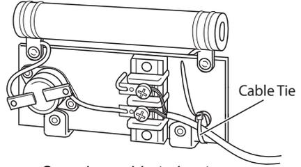
*Securing cable to heater*
