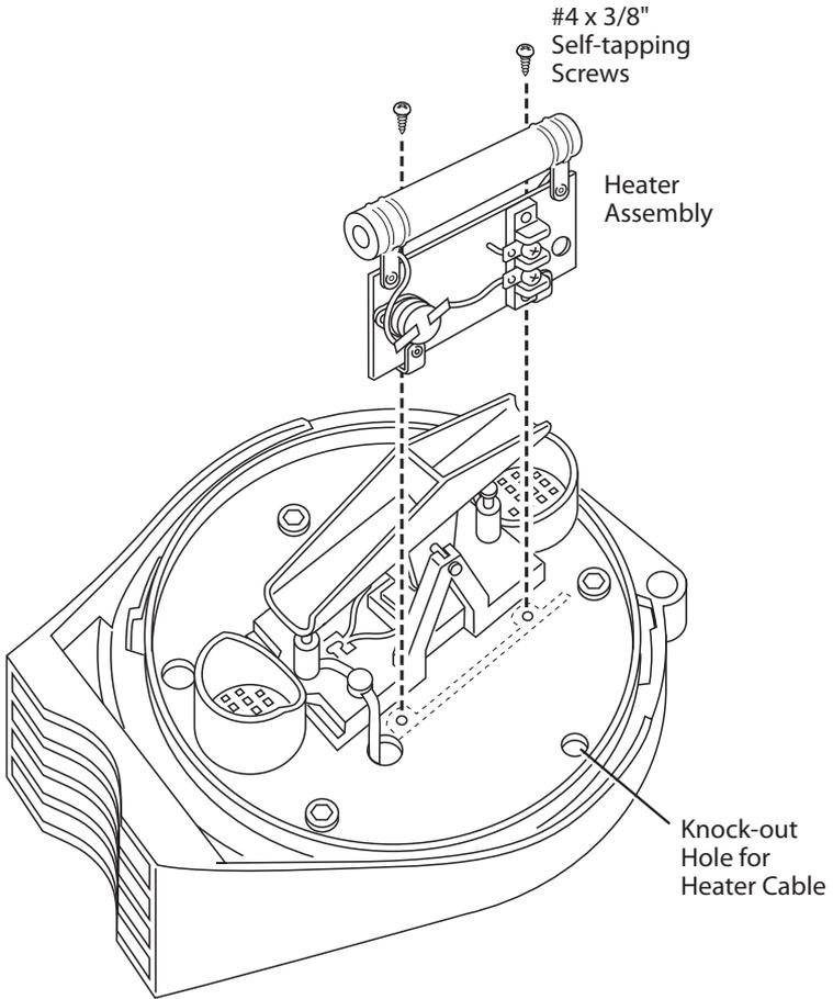
*Securing the heater in an Vantage Pro2 rain collector*
