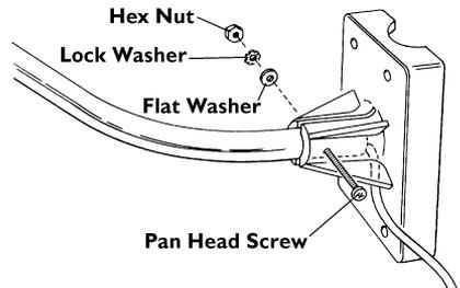
*Attaching the anemometer arm to the base*
