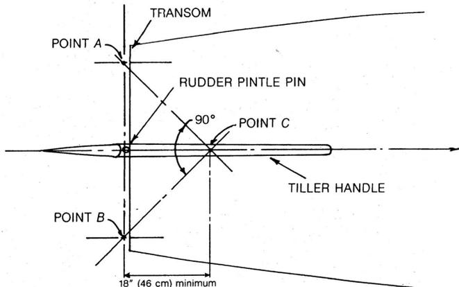
3. Assemble the Tiller-Tamer unit to the tiller handle by positioning the knob over point C. Attach with two wood screws provided. Release the knob and thread the 1/4" (6.4 mm) line through as shown below.
