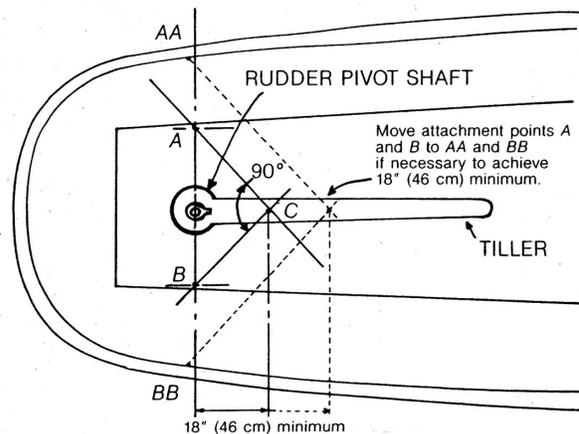
3. Assemble the Tiller-Tamer unit to the tiller handle by positioning the knob over point C. Attach with two wood screws provided. Release the knob and thread the 1/4" (6.4 mm) line through as shown below.
