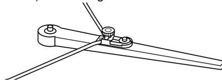
4. Use points A and B as cleat locations. Install clam cleats with fairleads (CL203 or CL211) as shown at right. Attach line at cleats as shown below.
