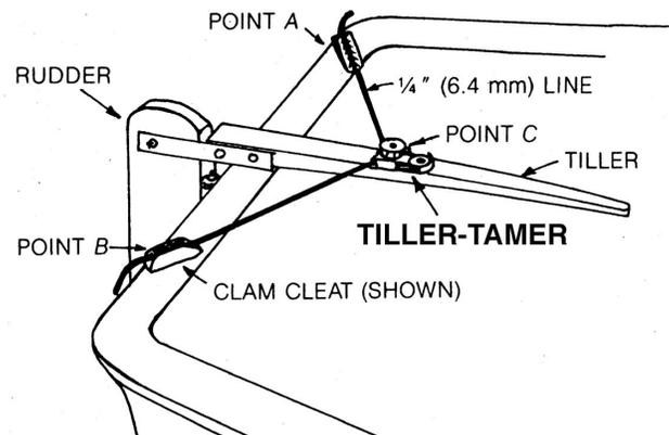
4. Attach a cleat at points A and B. This may be a clam cleat or any other quick releasing device. CL201 is recommended, as shown above.
