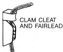
5. Attach one end of 1/4" (6.4 mm) line. With tiller amidships, loosen clamp knob on Tiller-Tamer. Pull line through to tension and attach to second clam cleat.
