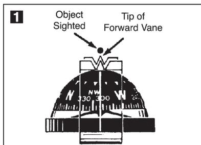
**Sighting Objects.** Hold the compass in a relaxed position at arms length, with the yellow cursor line facing you. With the compass slightly tipped so both pointers are visible, rotate your arm and upper body until both pointers are in-line with the object being sighted (figure 1). Read the magnetic bearing as it appears at the yellow cursor line.
